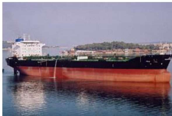
ULJANIK Tanker za ulje i kemikalije Tanker for oil and chemicals "Hispanica" 2x8L23/30H + 1x6L23/30H
